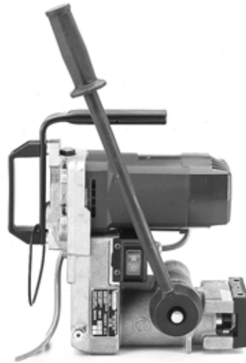
Ref. LD-2ENY: basic drill without clamping device
