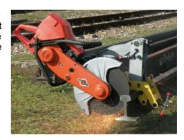
Designed for precise cutting, Robokatta Automatic Rail Disc Saw has the perfectly perpendicular action essential for making the consistently accurate right-angle cuts in both axes that are fundamental to the reliability of isolated joints in automatic signalling systems.
