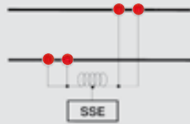
Return current connections to substations
